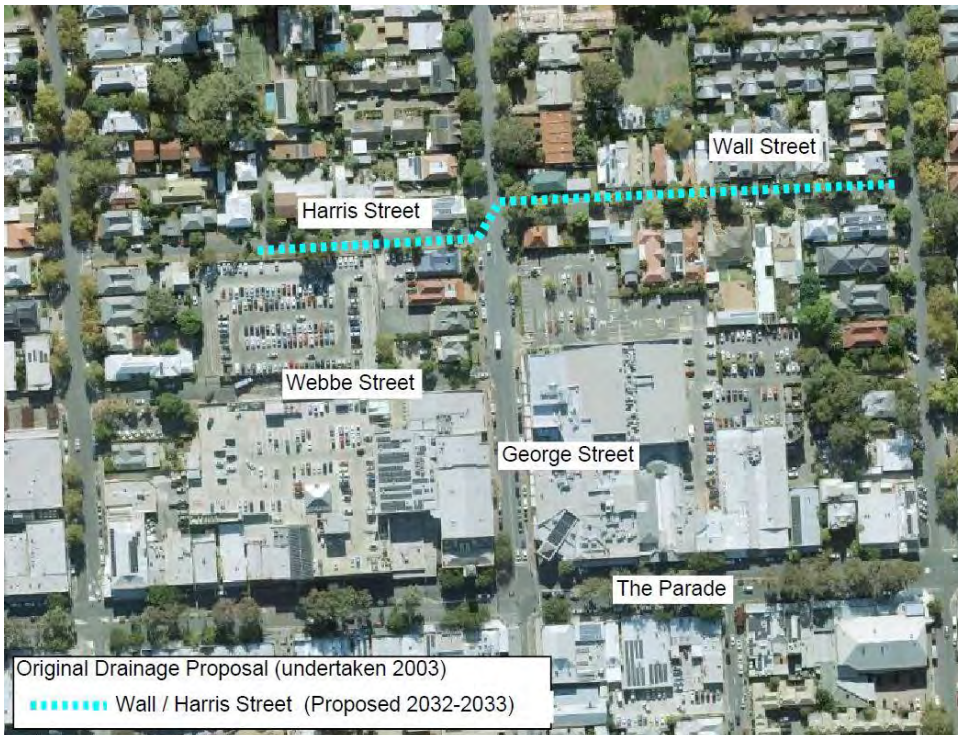
FIGURE 5: LONG TERM DRAINAGE PROGRAM – PROPOSED HARRIS STREET AND WALL STREET STORMWATER DRAINAGE WORKS 2003
