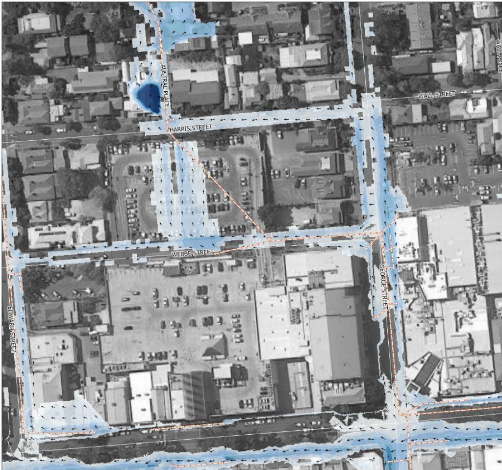
FIGURE 4: EXISTING CONDITIONS – 1% AEP FLOOD EVENT – THE PARADE TO GEORGE, EDWARD AND HARRIS STREET, NORWOOD
