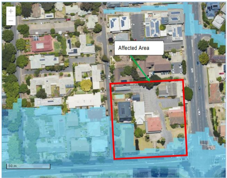
Figure 2: SA Government, Water Connect, Flood Awareness Map – Extract from the Gawler River Floodplain Mapping from 2015, 1 in 100 Chance Storm Event– Before Mitigation Works
